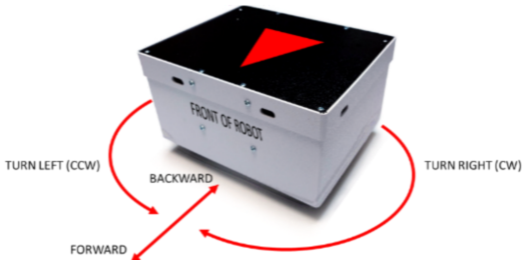
Figure 6-3 Directions of Robot Movement
